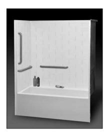
**Specification** – Oasis one-piece, 60 x 36-inch deep, FRP gelcoat flat wall bathtub model TST-6036 offered in a standard 16-inch or 17.25-inch (ABF) apron height. ActivLife package includes a single horizontal bar on the back wall and control wall, and a vertical bar at the entry on the control wall.
