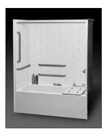
**Specification** – Oasis one-piece, 60 x 32-inch deep, FRP gelcoat flat wall bathtub model TST-6032 ABF (17.25-inch apron) having a factory-equipped package in compliance with ICC/ANSI A 117.1-2017. Package includes 2-horizontal bars on back wall, single horizontal bar on head end wall, horizontal bar on control wall, vertical bar at entry on control wall, pivot-hinge FOLDING in-tub seat at head end and shower curtain rod.
