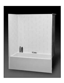
**Specification** – Oasis one-piece, 60 x 32-inch deep, FRP gelcoat flat wall bathtub model TST-6032, with a standard 17.25-inch (ABF) apron height. ActivLife package includes factory applied, 3-wall, mid-level reinforcement, exceeding (HUD/FHA) 'Fair Housing' requirements.
