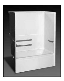
**Specification** – Oasis one-piece, 60 x 32-inch deep, FRP gelcoat flat wall bathtub model TSFW-6032 ABF with an 18.25-inch apron. ActivLife package includes 2-horizontal bars on back wall along with a single horizontal bar on head end wall and on the control wall.
