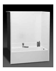
**Specification** – Oasis one-piece, 60 x 32-inch deep, FRP gelcoat flat wall bathtub model TSF-6032 ABF, having a 17.25-inch apron height. ActivLife package includes factory applied, 3-wall, mid-level reinforcement, exceeding (HUD/FHA) 'Fair Housing' requirements.
