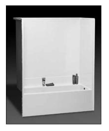
**Specification** – Oasis one-piece, 60 x 30-inch deep, FRP gelcoat flat wall bathtub model TSF-6030 ABF, having a 17.25-inch apron height. ActivLife package includes factory applied bars only reinforcement package, in compliance with HUD/FHA Fair Housing Act Design Manual. Listed reinforcement only package includes areas for 2-horizontal bars on back wall, a single horizontal bar on head end wall, a single horizontal bar on control wall.
