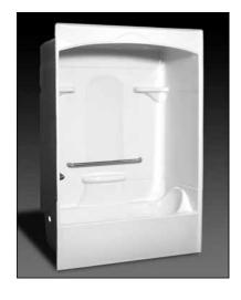
**Specification** – Oasis one-piece, 60 x 32-3/4-inch deep, vacuum formed acrylic bathtub with integral unit dome, model TSA-DM-6033, offered in a standard 16-inch or 17.25-inch (ABF) apron height. ActivLife package includes a horizontal bar on the back wall and across the control wall.
