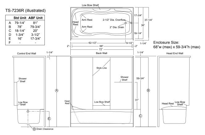
Sump Dimensions: 58" long x 21" wide x 15-3/4" deep / Sump Capacity: 65 gal. (unoccupied - to overflow)
