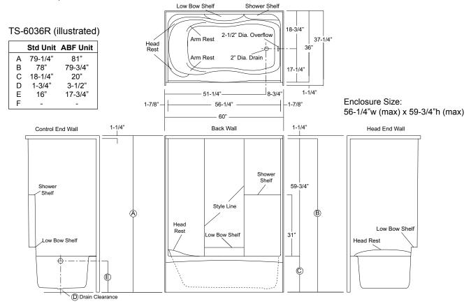
Sump Dimensions: 46-1/2" long x 20-3/4" wide x 15-3/4" deep / Sump Capacity: 60 gal. (unoccupied - to overflow) Whirlpool Operating: 45 gal.
