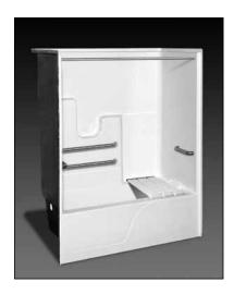
**Specification** – Oasis one-piece, 60 x 32-inch deep, FRP gelcoat bathtub model TS-6032 ABF (17.25-inch apron) having a factory-equipped package in compliance with 2010 ADA Standards for Accessible Design. Package includes 2-horizontal bars on back wall, single horizontal bar on head end wall, horizontal bar on control wall, REMOVABLE in-tub seat at head end and shower curtain rod.
