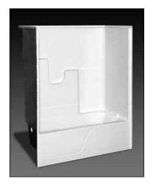
**Specification** – Oasis one-piece, 60 x 32-inch deep, FRP gelcoat bathtub model TS-6032, offered in a standard 16-inch or 17.25-inch (ABF) apron height. ActivLife package includes factory applied, 3-wall, full-wrap reinforcement, exceeding (HUD/FHA) 'Fair Housing' requirements.
