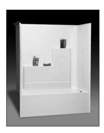
**Specification** – Oasis one-piece, 60 x 30-inch deep, FRP gelcoat bathtub model TS-6030, offered in a 17.25-inch (ABF) apron height. ActivLife package includes factory-applied bars only reinforcement package, in compliance with HUD/FHA Fair Housing Act Design Manual. Listed reinforcement only package includes areas for 2-horizontal bars on back wall, a single horizontal bar on head end wall, a single horizontal bar on control wall, and a single vertical bar at entry on control wall.
