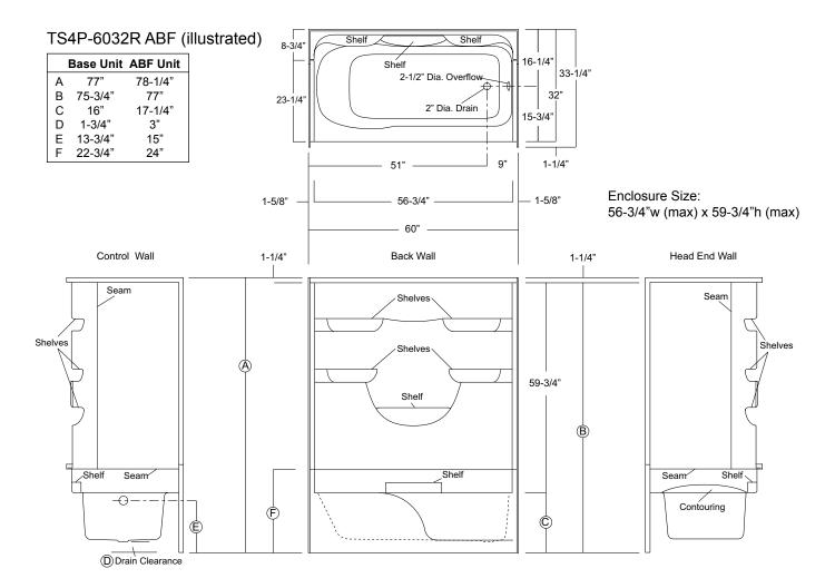
Sump Dimensions: 51" long x 22" wide x 13-1/4" deep Sump Capacity: 42 gal. (unoccupied - to overflow)
