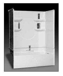
**Specification** – Oasis 4-piece, 60 x 30-inch deep, FRP gelcoat bathtub model TS4P-6030 with a 17.25-inch (ABF) apron height. ActivLife package includes factory applied bars only reinforcement package, in compliance with HUD/FHA Fair Housing Act Design Manual. Listed reinforcement only package includes areas for 2-horizontal bars on back wall, a single horizontal bar on head end wall, a single horizontal bar on control wall, and a single vertical bar at entry on control wall.
