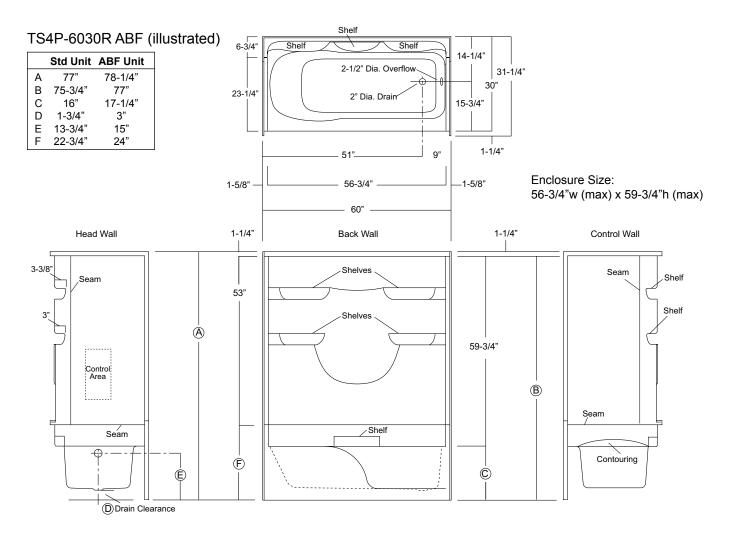
Sump Dimensions:51" long x 20" wide x 13-1/4" deepSump Capacity:40 gal. (unoccupied - to overflow)
