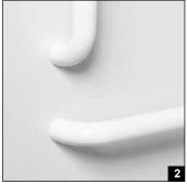
Photo 1: Grab Bars: Factory-installed 1.50-inch dia. stainless steel, concealed attachment, 18 gauge, #304 brushed stainless steel grab bars. Concealed attachment design provides tamper-resistance and minimizes debris collection areas at contact points, compared to common exposed flange bar designs, without compromising bar attachment integrity. (Reinforced areas include a structural core material encapsulated in FRP composite.)
