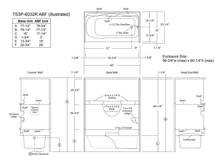
Sump Dimensions: 51" long x 22" wide x 13-1/4" deep Sump Capacity: 42 gal. (unoccupied - to overflow)
