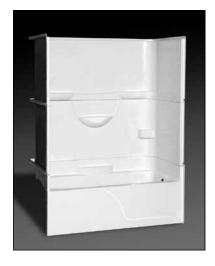
**Specification** – Oasis 3-piece, 60 x 30-inch deep, FRP gelcoat bathtub model TS3P-6030 with a 17.25-inch (ABF) apron height. ActivLife package includes factory applied bars only reinforcement package, in compliance with HUD/FHA Fair Housing Act Design Manual. Listed reinforcement only package includes areas for 2-horizontal bars on back wall, a single horizontal bar on head end wall, a single horizontal bar on control wall, and a single vertical bar at entry on control wall.
