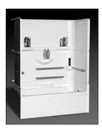
**Specification** – Oasis 3-piece, 60 x 30-inch deep, FRP gelcoat bathtub model TS3P-6030, offered in a standard 16-inch or 17.25-inch (ABF) apron height. ActivLife package includes 2-horizontal bars on back wall along with a single horizontal bar on head end wall and on the control wall.
