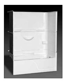
**Specification** – Oasis 3-piece, 60 x 30-inch deep, FRP gelcoat bathtub model TS3P-6030 with a 17.25-inch (ABF) apron height. ActivLife package includes factory applied, 3-wall, mid-level reinforcement, exceeding (HUD/FHA) 'Fair Housing' requirements.
