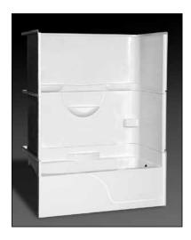
**Specification** – Oasis 3-piece, 60 x 30-inch deep, FRP gelcoat bathtub model TS3P-6030 with a 17.25-inch (ABF) apron height. ActivLife package includes factory applied, 3-wall, full-wrap reinforcement, exceeding (HUD/FHA) 'Fair Housing' requirements.
