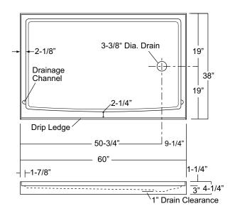
NOTE: Critical enclosure dimensions should be taken directly from the installed shower base with finished wall surround.
