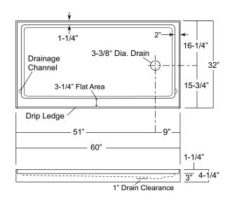
NOTE: Critical enclosure dimensions should be taken directly from the installed shower base with finished wall surround.
