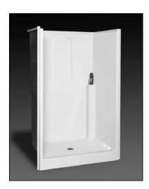
**Specification** – Oasis one-piece FRP gelcoat shower compartment SH-WX-4838, with an expanded shower entry profile to minimize transfer space into the shower, offered in a standard 4-inch or 6-inch (ABF) dam configuration. ActivLife package includes factory applied, 3-wall, full-wrap reinforcement, exceeding (HUD/FHA) 'Fair Housing' requirements.
