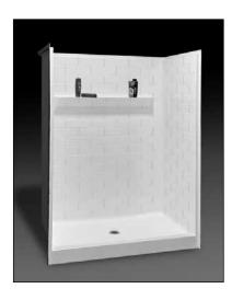
**Specification** – Oasis one-piece FRP gelcoat shower compartment SHT-6034, offered in a standard 3-inch or 5-inch (ABF) dam configuration. ActivLife package includes factory applied, 3-wall, mid-level wrap reinforcement, exceeding (HUD/FHA) 'Fair Housing' requirements.
