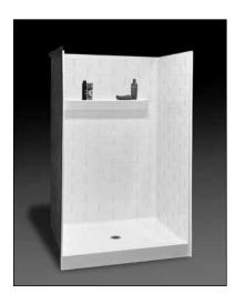
**Specification** – Oasis one-piece FRP gelcoat shower compartment SHT-5038, offered in a standard 3-inch or 5-inch (ABF) dam configuration. ActivLife package includes factory applied, 3-wall, mid-level wrap reinforcement, exceeding (HUD/FHA) 'Fair Housing' requirements.
