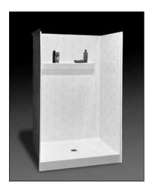
**Specification** – Oasis one-piece FRP gelcoat shower compartment SH-5038, offered in a standard 3-inch or 5-inch (ABF) dam configuration. ActivLife package includes factory applied, 3-wall, full-wrap reinforcement, exceeding (HUD/FHA) 'Fair Housing' requirements.
