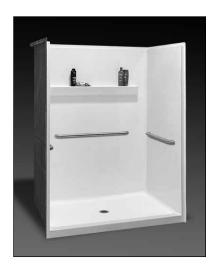
**Specification** – Oasis one-piece FRP gelcoat shower compartment SHS-6038, offered in a standard 3-inch or 5-inch (ABF) dam configuration. ActivLife package includes a single horizontal bar on the back wall and single horizontal bars on each side wall..
