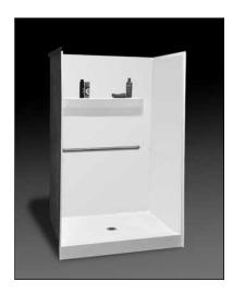
**Specification** – Oasis one-piece FRP gelcoat shower compartment SHS-5038, offered in a standard 3-inch or 5-inch (ABF) dam configuration. ActivLife package includes a single horizontal bar on the back wall.
