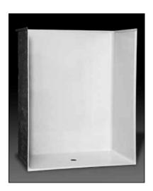
**Specification** – Oasis one-piece FRP gelcoat shower compartment SHMT-6238, having a 60 x 36-inch minimum clear interior dimension and ½-inch high maximum finished threshold with floor attachment flange on lower threshold. An ActivLife factory-applied reinforcement only package, in compliance with HUD/FHA Fair Housing Act Design Manual, shall include back wall and both side wall reinforcement for horizontal bar application.
