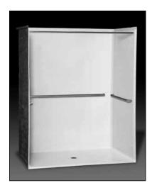
**Specification** – Oasis one-piece FRP gelcoat shower compartment SHMT-6238, having a 60 x 36-inch minimum clear interior dimension and  $\frac{1}{2}$ -inch high maximum finished threshold with floor attachment flange on lower threshold. A factory-equipped package, in compliance with 2010 ADA Standards & ICC/ANSI A117.1-2017 for Accessible Design, shall include horizontal bars across each side wall and back wall and a shower curtain rod.
