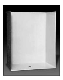
**Specification** – Oasis one-piece FRP gelcoat shower compartment SHMT-6238, having a 60 x 36-inch minimum clear interior dimension and  $\frac{1}{2}$ -inch high maximum finished threshold with floor attachment flange on lower threshold. ActivLife package includes factory applied, 3-wall, mid-level wrap reinforcement, exceeding (HUD/FHA) 'Fair Housing' requirements.
