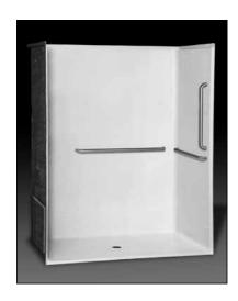
**Specification** – Oasis one-piece FRP gelcoat shower compartment SHMT-6238, having a 60 x 36-inch minimum clear interior dimension and ½-inch high maximum finished threshold with floor attachment flange on lower threshold. An ActivLife factory-equipped package, in compliance with ICC/ANSI A117.1-2017 for Accessible Design, shall include a horizontal and vertical bar on the side wall opposite the seat, a horizontal bar on the back wall and seat reinforcement opposite the control wall.
