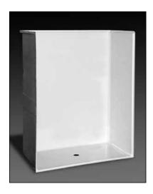
**Specification** – Oasis one-piece FRP gelcoat shower compartment SHMT-6232, having a 60 x 30-inch minimum clear interior dimension and  $\frac{1}{2}$ -inch high maximum finished threshold with floor attachment flange on lower threshold. An ActivLife factory-applied reinforcement only package, in compliance with HUD/FHA Fair Housing Act Design Manual, shall include back wall and both side wall reinforcement for horizontal bar application.
