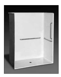
**Specification** – Oasis one-piece FRP gelcoat shower compartment SHMT-6232, having a 60 x 30-inch minimum clear interior dimension and ½-inch high maximum finished threshold with floor attachment flange on lower threshold. An ActivLife factory-equipped package, in compliance with ICC/ANSI A117.1-2017 for Accessible Design, shall include a horizontal bar across the control wall and back wall, vertical bar on the control wall and seat reinforcement opposite the control wall.
