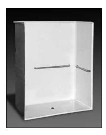
**Specification** – Oasis one-piece FRP gelcoat shower compartment SHMT-6232, having a 60 x 30-inch minimum clear interior dimension and  $\frac{1}{2}$ -inch high maximum finished threshold with floor attachment flange on lower threshold. An ActivLife factory-equipped package, in compliance with ICC/ANSI A117.1-2009 for Accessible Design, shall include a horizontal bar across the control wall and back wall with seat reinforcement opposite the control wall.
