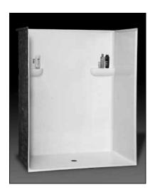
**Specification** – Oasis one-piece FRP gelcoat shower compartment SHMD-6238, having a 60 x 36-1/2-inch minimum clear interior dimension and ½-inch high maximum finished threshold with floor attachment flange on lower threshold. An ActivLife factory-equipped package shall include 2-wall horizontal and single-wall vertical bar reinforcement and seat reinforcement.
