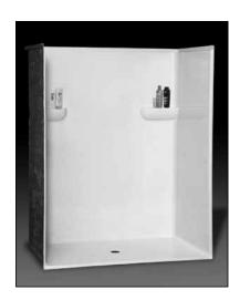
**Specification** – Oasis one-piece FRP gelcoat shower compartment SHMD-6238, having a 60 x 36-1/2-inch minimum clear interior dimension and ½-inch high maximum finished threshold with floor attachment flange on lower threshold. ActivLife package includes factory applied, 3-wall, mid-level wrap reinforcement, exceeding (HUD/FHA) 'Fair Housing' requirements.
