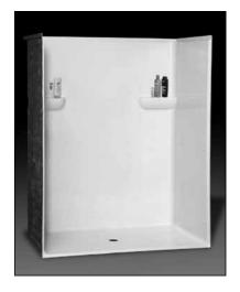
**Specification** – Oasis one-piece FRP gelcoat shower compartment SHMD-6238, having a 60 x 36-1/2-inch minimum clear interior dimension and ½-inch high maximum finished threshold with floor attachment flange on lower threshold. ActivLife package includes factory applied, 3-wall, full-wrap reinforcement, exceeding (HUD/FHA) 'Fair Housing' requirements.
