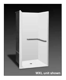
Specification - Oasis one-piece FRP gelcoat shower compartment SHFW-WXR/L-3837, having a 36 x 36-inch clear interior dimension. <sup>1</sup>/<sub>2</sub>-inch high maximum finished threshold with floor attachment flange on lower threshold, and a single R or L expanded shower entry wall reveal to minimize transfer space. An ActivLife factory-equipped package shall include a horizontal interior corner bar across control wall and on back wall, and reinforcement for seat opposite control wall.
