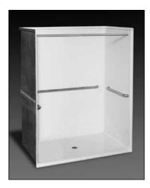
**Specification** – Oasis one-piece FRP gelcoat shower compartment SHFW-6235, having a 60 x 30-inch minimum clear interior dimension and 7/16-inch high maximum finished threshold with floor attachment flange on lower threshold. A factory-equipped package, in compliance with 2010 ADA Standards & ICC/ANSI A117.1-2017 for Accessible Design, shall include a horizontal bar across each side wall and back wall and shower curtain rod.
