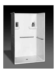
**Specification** – Oasis one-piece FRP gelcoat shower compartment SHFW-5038, having a 1/2-inch high maximum finished, ramped threshold with floor attachment flange on lower threshold. ActivLife package includes a single horizontal bar on the back wall and control wall.
