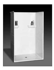
**Specification** – Oasis one-piece FRP gelcoat shower compartment SHFW-5038, having a 1/2-inch high maximum finished, ramped threshold with floor attachment flange on lower threshold. ActivLife package includes factory applied, 3-wall, full-wrap reinforcement, exceeding (HUD/FHA) 'Fair Housing' requirements.
