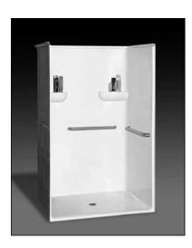
**Specification** – Oasis one-piece FRP gelcoat shower compartment SHFW-4836, having a 1/2-inch high maximum finished, ramped threshold with floor attachment flange on lower threshold. ActivLife package includes a single horizontal bar on the back wall and control wall.
