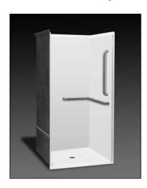
**Specification** – Oasis one-piece FRP gelcoat shower compartment SHFW-3837, having a 36 x 36-inches clear interior dimension and ½-inch high maximum finished threshold with floor attachment flange on lower threshold. An ActivLife factory-equipped package shall include a horizontal interior corner bar across the control wall and on back wall, a single <u>vertical bar at entry on control wall</u>, and reinforcement for seat opposite control wall.
