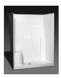
**Specification** – Oasis one-piece FRP gelcoat shower compartment SH-6036 RS or LS, having a single contoured seat and offered in a standard 4-inch or 6-inch (ABF) dam configuration. ActivLife package includes factory-applied reinforcement, in compliance with HUD/FHA Fair Housing Act Design Manual, on back wall and control wall opposite seat for horizontal bar application.
