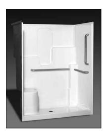
**Specification** – Oasis one-piece FRP gelcoat shower compartment SH-6036 RS or LS, having a single contoured seat and offered in a standard 4-inch or 6-inch (ABF) dam configuration. ActivLife package includes a horizontal bar across the back wall, a bar across the control wall, and a vertical bar at the entry on the control wall.
