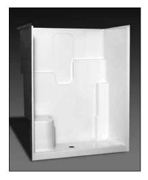
**Specification** – Oasis one-piece FRP gelcoat shower compartment SH-6036 RS or LS, having a single contoured seat and offered in a standard 4-inch or 6-inch (ABF) dam configuration. ActivLife package includes factory applied, 3-wall, mid-level wrap reinforcement, exceeding (HUD/FHA) 'Fair Housing' requirements.
