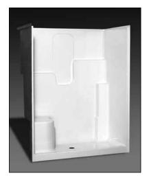
**Specification** – Oasis one-piece FRP gelcoat shower compartment SH-6036 RS or LS, having a single contoured seat and offered in a standard 4-inch or 6-inch (ABF) dam configuration. ActivLife package includes factory applied, 3-wall, full-wrap reinforcement, exceeding (HUD/FHA) 'Fair Housing' requirements.
