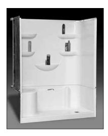
**Specification** – Oasis 4-piece FRP gelcoat shower compartment, SH4P-6032 RS or LS, having a single contoured seat and offered in a standard 4-inch or 6-inch (ABF) dam configuration. ActivLife package includes factory-applied reinforcement, in compliance with HUD/FHA Fair Housing Act Design Manual, for 2-horizontal bars on back wall, a single horizontal bar on head end wall, a single horizontal bar on control wall, and vertical bars at entry on both side walls.
